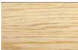
**VBQ** : Finger jointing every 0,80m minimum, width up to 100mm without splicing, up to 300mm with splicing.
